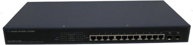
**Waters Network Systems' GSM PoE models** provide 12 10/100/1000Base-TX ports for your wiring closet or small workgroups with two optional mini GBIC slots for fiber Gigabit connectivity. PoE ports provide power to end devices such as wireless access points or VoIP phones directly through existing LAN cables. Waters' GSM series provides a cost savings migration path from 10 to 1000Mbps switched Ethernet.
