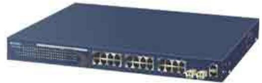
**Waters Network Systems' ProSwitch 2126M-PoE model** provides 24 10/100Base-TX ports for your wiring closet with two mini GBIC slots for fiber or copper Gigabit connectivity. PoE ports provide power to end devices such as wireless access points, VoIP phones or security cameras directly through existing LAN cables. Waters' Gigabit switch provides a cost savings migration path from 10 to 1000Mbps switched Ethernet.
