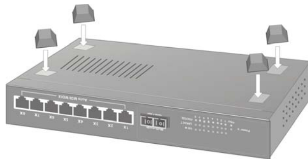
Figure 3-6. Attaching Rubber Feet to each corner on the bottom of the switch
