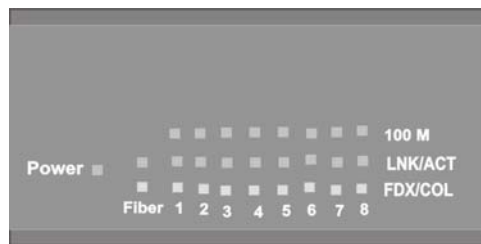
Figure 3-5. LED Indicators for 1008 Switch
