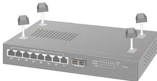
Figure 3-5. Attaching Rubber Feet to each corner on the bottom of the Switch
