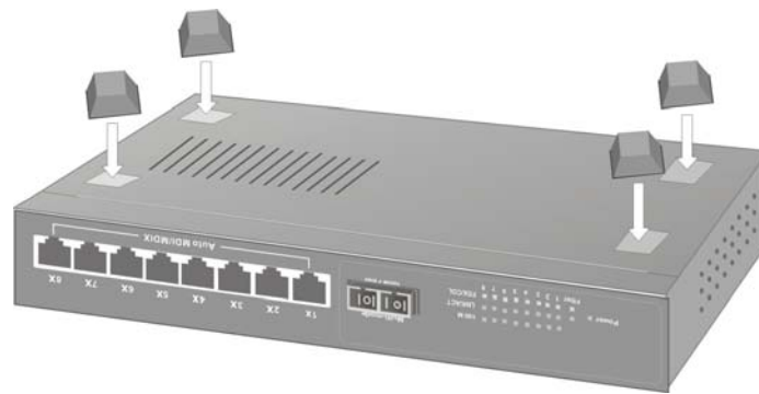
Figure 3-8. Attaching Rubber Feet to each corner on the bottom of the switch
