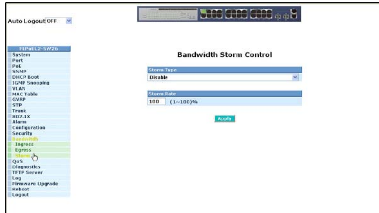
Figure 5.63 – Bandwidth Storm Control
