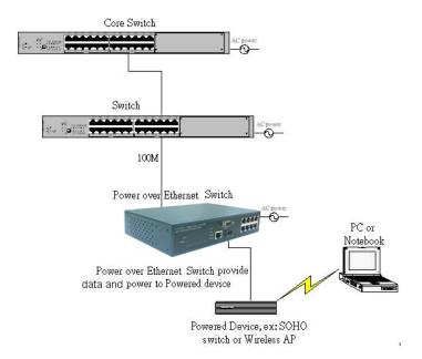
Figure 4.3 – PoE Switch with Wireless Powered Device
