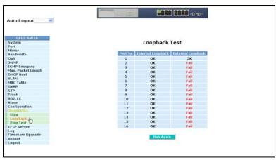
Figure 5.70 - Loopback Test
