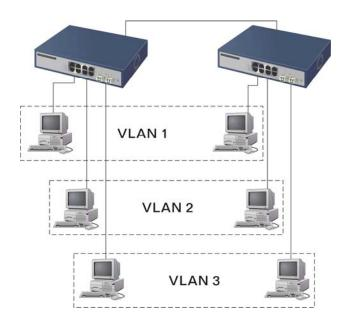
Figure 3-7 Attribute-based VLAN Diagram
