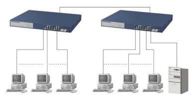
Figure 3.4 - No VLAN Configuration Diagram
