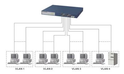
Figure 3.5 - Port-based VLAN Diagram
