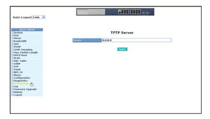
Figure 5.72 – TFTP Server Assignment
