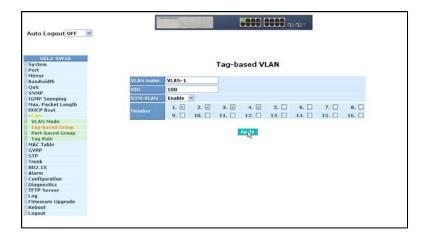
Figure 5.32 - Tag-based VLAN
