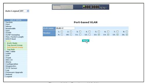
Figure 5.35 - Port-based VLAN
