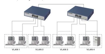
Figure 3-6 - Port-based VLAN Diagram
