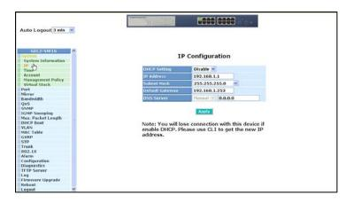
Figure 5.4 - IP Address Configuration
